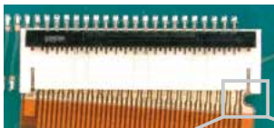
Incomplete FPC insertion
